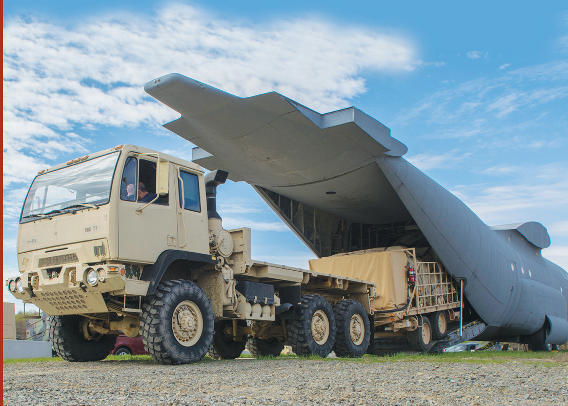
Tobyhanna Army Depot personnel load the Integrated Air and Missile Defense trailer onto a C-130 Hercules aircraft mockup to verify all clearance requirements are met.
